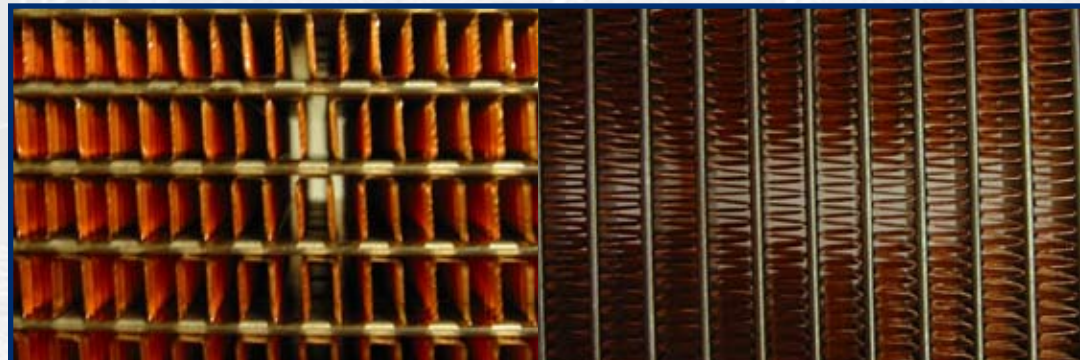
Corrugated fins are replacing conventional plate fins in locomotive applications. The rectangular or square wave fins (left) are preferred over the triangular fins (right) for use in harsh environments because they are easier to clean.
