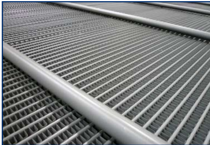
Close-up of a CuproBraz e CAC built for a locomotive application. Note that the copper fins and brass tubes have been painted. New emissions standards for locomotives will be discussed in Part II. (Photograph is courtesy of Young Touchstone.)
