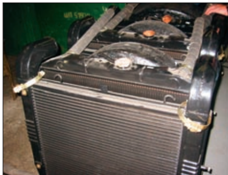
CuproBrazed heat-exchangers are ready for mounting in URAL trucks. SHAAZ integrates the charge air cooler and radiator into a single package before delivery to URAL. The integrated package can be quickly and easily mounted into the engine compartment at the URAL plant.
