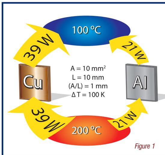
Copper clearly conducts more heat per unit volume than aluminum. For heat exchanger designs, this directly impacts what is sometimes called heat-transfer efficiency. For identical geometries, a copper element will remove more heat compared to aluminum. Valtra Inc. uses copper-and-brass charge air coolers in many of its tractor designs mainly because of this size advantage. The CAC fits better in the tractor because of its reduced size and the design affords better visibility to the operator.
