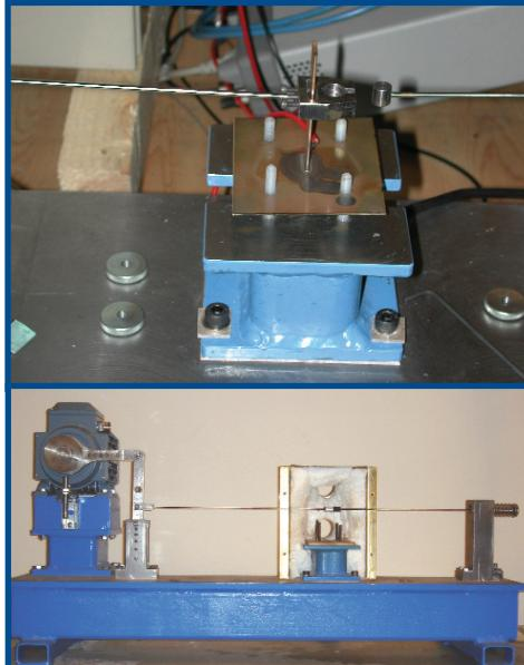
The tube specimen is mounted on a fixture (top), which can be enclosed by a heater (bottom).
