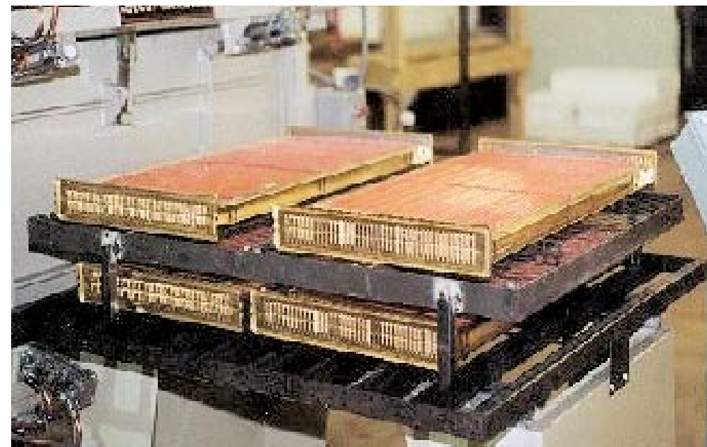
A double layer of radiators is being brazed in a CuproBrazed furnace.
