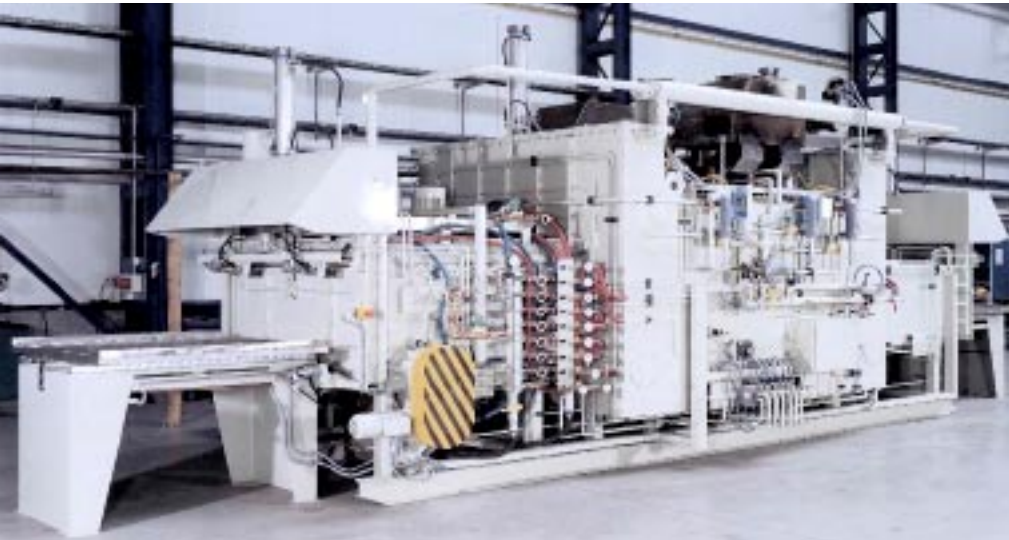
Many manufacturers prefer a semi-continuous, three-chamber furnace for intermediate volume production. (Furnace built by SECO/ WARWICK.)
