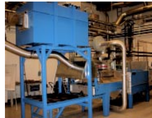
The CuproBrazed center in Västerås, Sweden employs a batch furnace in the production of prototype heat exchangers. (Furnace built by Sarlin.)
