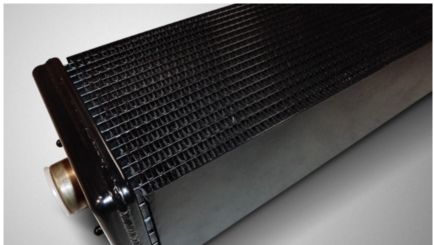
Fig. 2. Coated mid-size radiator with six tube rows. The black appearance of the tubes on the cross section in the right demonstrates the complete penetration of the coating through the core.
