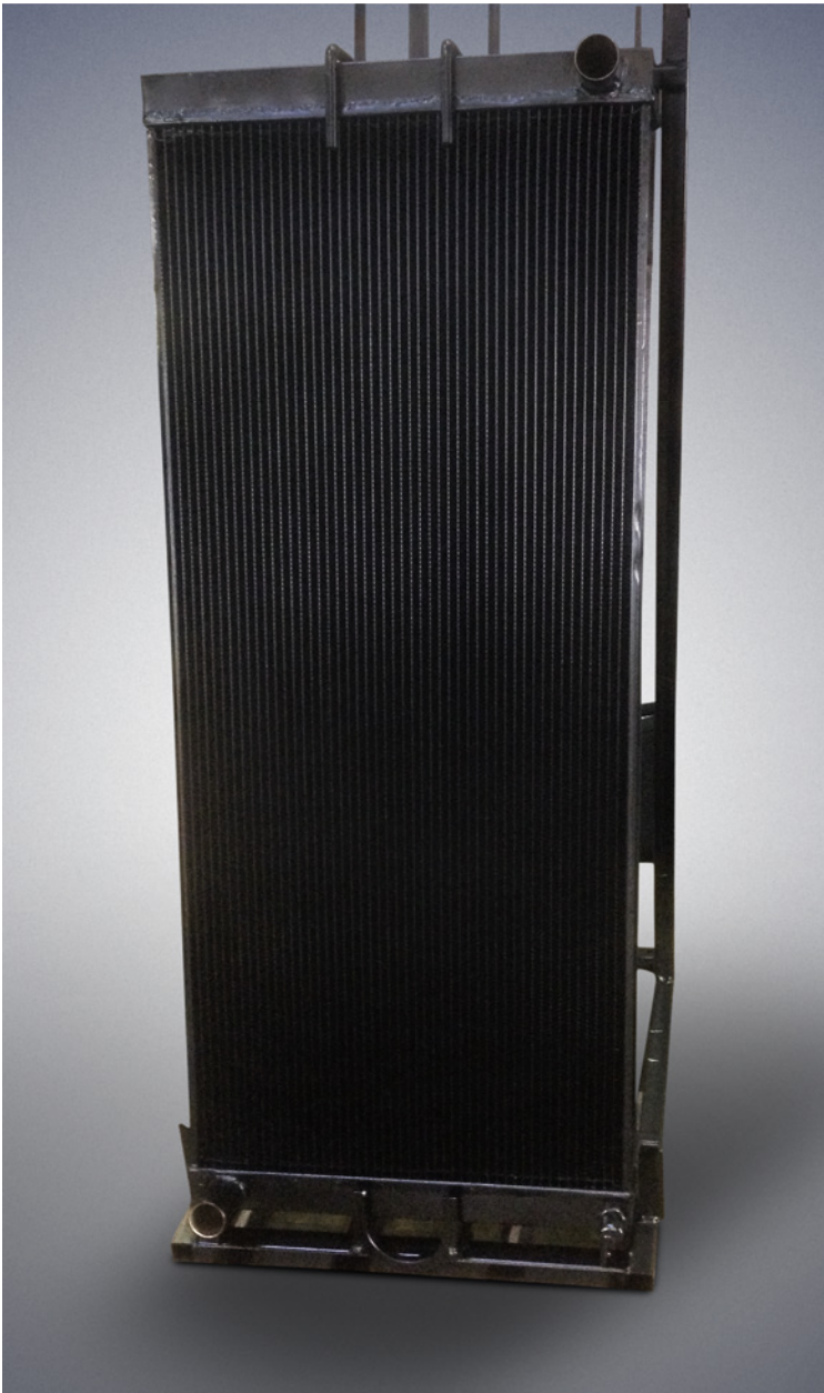
Fig. 7. Full size DuraFin™ radiator on the coating rack designed for a mining vehicle
